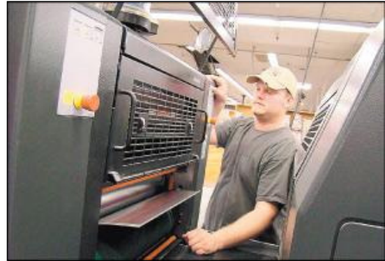
JOSEPH LAW/Standard Journal -- Kelly Hansen, a pressman at Artco, loads the printing plate in the company's new Heidelberg Anicolor press.
